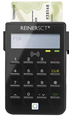
FIG. 3. Standard Reader: cyberJack RFID standard (USB)
